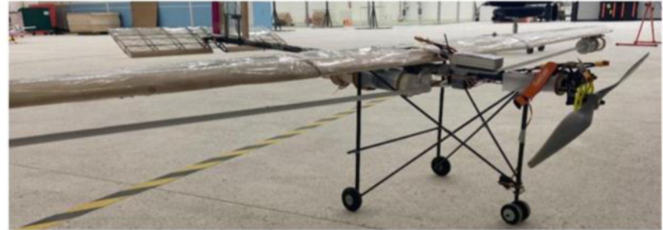
(a) Lateral water-driven moving-mass demonstrator installation
